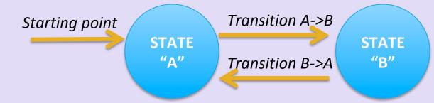
An FSM is defined by a list of its states, its initial state, and the conditions for each transition.
