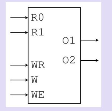
*This will be made from D-FFs or D-Latches and Combinatorial Logic*
